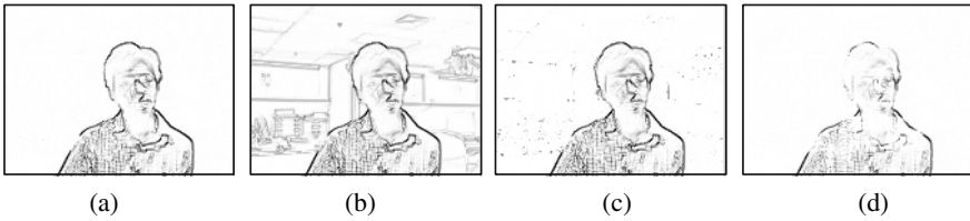
Fig. 5. Parameter settings. (a) K = 5, \sigma_z = 10 . (b) K = 500, \sigma_z = 10 . (c) K = 5, \sigma_z = 1 . (d) K = 5, \sigma_z = 50 .
