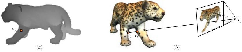
Fig. 3. For the visibility estimation of a voxel v in image I_j we first store the depth values of all backfacing voxels v_b in a depth map T_d (a). The visibility of each v can then be evaluated by a depth comparison of v and the corresponding entry in T_d (b).
