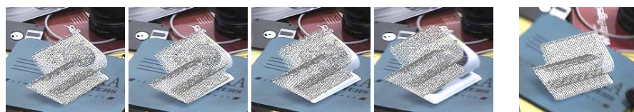
Fig. 7. Accumulation of errors when only flow based correspondences are used. From Left to Right: Pose results at frames 2, 5, 10, and 20. Rightmost: Pose result at frame 242 if contour and flow based correspondences are employed.
