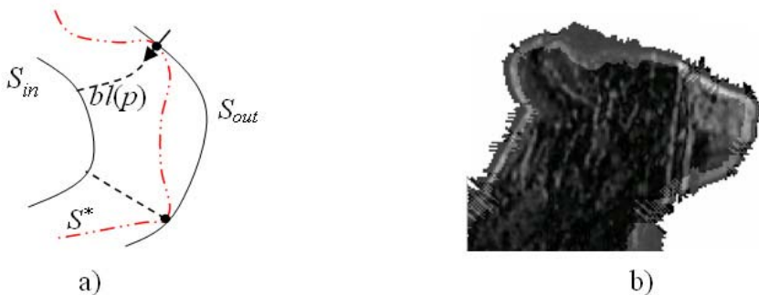
Fig. 3. a) Blocking regions (curves). b) Locational uncertainties (gray areas) of the contour extracted from a difference image.
