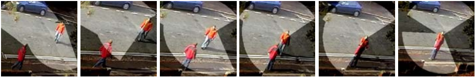
Fig. 7. Two people meeting could potentially be identified by each person being in the other’s gaze (in addition to other cues such as proximity), as we show in this example
