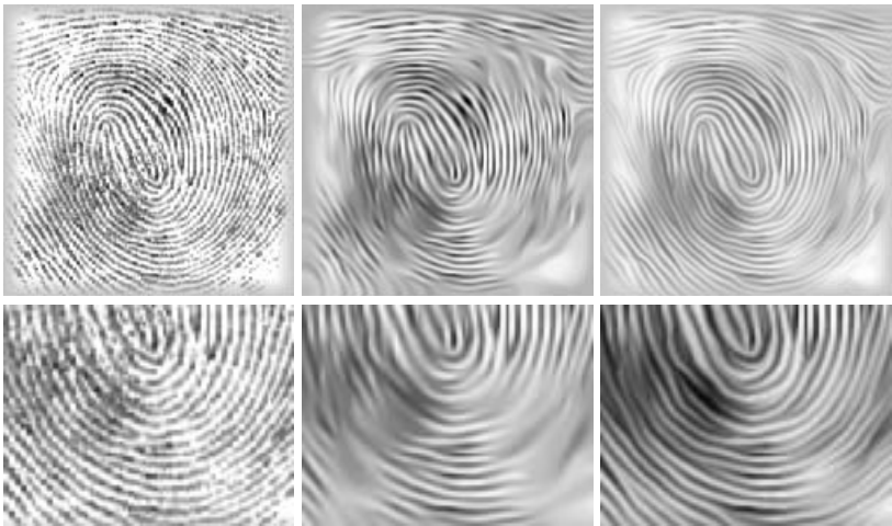
(a) Image of a fingerprint (b) Applying trace-based PDE (4), with p_1 = 0.5, p_2 = 1.2 . (c) Applying our constrained PDE (11), with p_1 = 0.5, p_2 = 1.2 .
