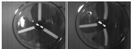
Fig. 1. An example of distortion of a rotating ventilator observed with a Rolling Shutter camera: static object (right image) and moving object (left image)
